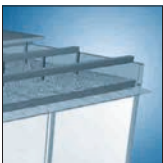
Ceiling with mineral wool insulation (40 mm thick)
